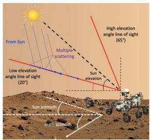
Fig. 1. Geometry of the passive sky observation.
