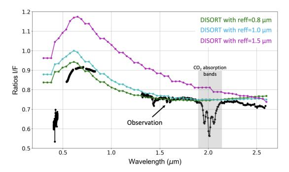
Fig. 2. Mean ratio of the low elevation spectra to the high elevation spectra. Black points are observations for sol 133 (solar longitude Ls=68°). DISORT model results are shown for different choices of dust particle sizes. The model matches the near-infrared data relatively well using 0.8-1 µm dust particles. However, the UV-VIS data are not well reproduced. We are currently investigating this issue.
