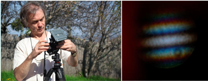
Figure 62. Solar fringes photographed with an EOS 5D Canon camera in front of which was set a micro-interferometer consisting of two holes having a diameter of 11.8 \mu separated by a baseline of 29.4 \mu .
