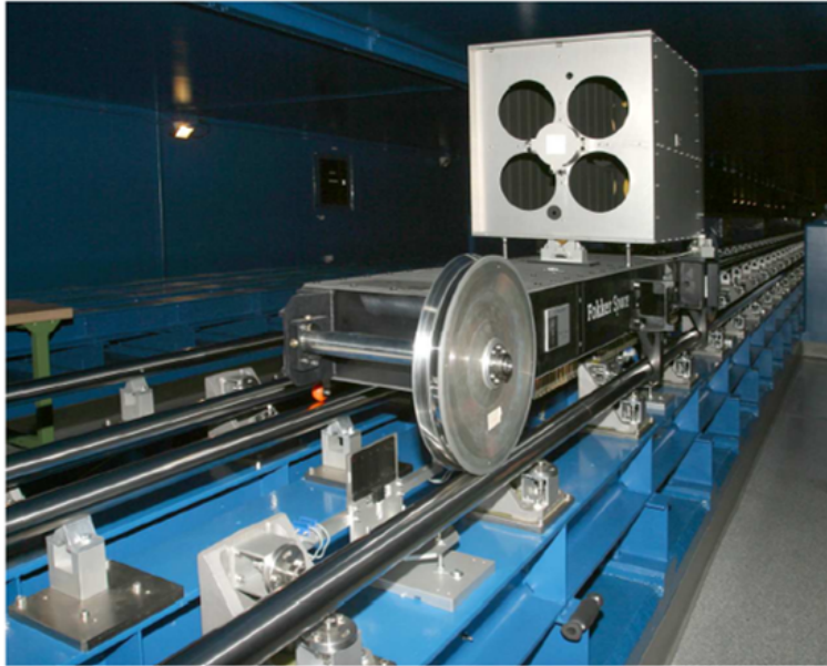
Figure 94. One of the VLTI delay line installed on its rails and supporting the cat's eye.
