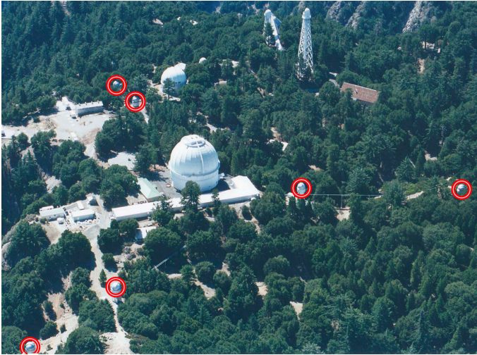
Figure 69. The CHARA interferometer composed of six 1m telescopes at Mount Wilson Observatory (California, USA). © The Observatories of the Carnegie Institution.
